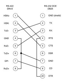
This cable is commonly referred to as a "hardware handshaking cable". In this arrangement, the TxD+ pin is not used, which is OK because the RS-232 device will detect incoming signals on the basis of the voltage difference between TX and ground. On the other hand, the Mac needs to measure the voltage between its RxD- and RxD+ pins, so the RxD+ pin is connected to the RS-232 ground.
