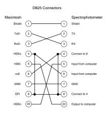
This results in lots of pins being connected together: Pins 4, 6 and 8 on each side are all tied together. I'm not sure exactly why this works, but it seems likely that Pin 4 or 8 on the spectrophotometer side needs a handshaking signal from the computer side.
