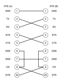
Because the handshaking pins are connected between the two devices, there is at least the potential for hardware control, provided that the two devices treat the connections properly. With this type of connection, the RTS signal of one device, say A, cannot play its usual role of activating the receiver of the other device, since it is now connected to the CTS pin of device B, which would normally be interpreted as an "OK to transmit signal" for B.
