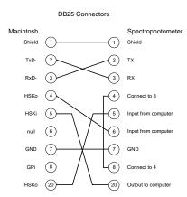
Some additional jumpers can be added to make the connector symmetrical:
