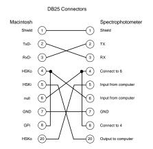
These additions are not likely to have any functional consequences. Pin 6 on the computer side is not connected to anything, and Pin 8 on the computer side is the GPi pin, which is an input but is not usually needed. Notice that this set of connections is exactly like the ones specified in the manufacturer's cable!
