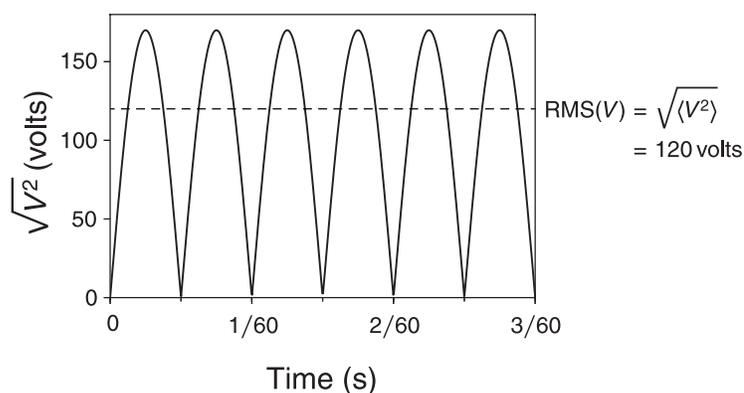
Notice that the peaks in the plot have slightly different shapes than those in the plot of  $V^2$ , and the peaks have a height of 170 V. The RMS average over time is 120 V, and it is this average that is usually specified for AC circuits. Note that the RMS average is calculated as the square root of the mean-square average and *not* by averaging over the square root of the squares of the individual values, which would, in general, give a different result.
