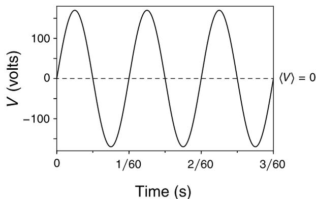
Note that the voltage oscillates between a maximum of 170 V and a minimum of  $-170$  V, with the average over time being 0 V. For the US power system, each cycle takes  $1/60$  s, for a frequency of 60 Hz. Although mathematically correct, the simple average of the voltage over time obviously doesn't convey much information about the power available from the current. To obtain a positive value, the instantaneous voltage can be squared to generate the plot below.
