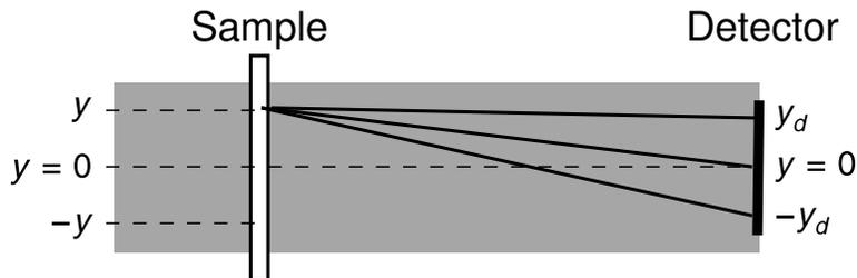
Figure 1.10: Effect of detector position,  $y_d$ , on effective scattering angle.
