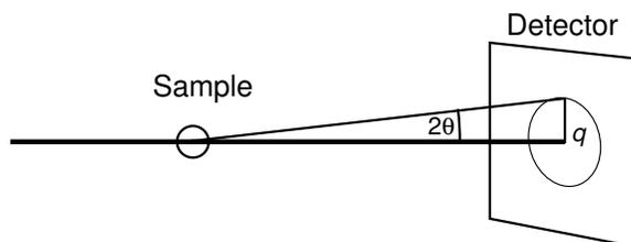
Figure 1.2: A SAXS camera with a point-collimated beam and a two-dimensional detector
