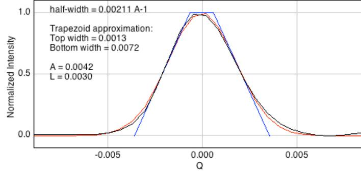
Figure 1.9: A fit of trapezoidal and Gaussian functions to a measured beam-width profile. From ImageJ with the saxsess plugin.
