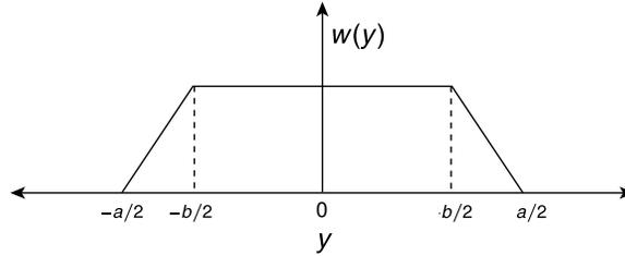
Figure 1.7: trapezoidal weighting function for the beam length profile.
