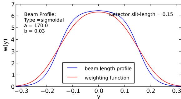
Figure 1.13: Weighting function for a sigmoidal beam profile, with (red) and without (blue) additional smearing due to integration over a detector slit width of  $0.15 \text{ \AA}^{-1}$
