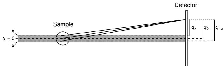
Figure 1.5: Contribution of X-rays scattered from multiple points along the beam width to the intensity detected at point  $q_0$ .
