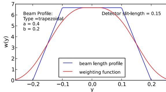
Figure 1.12: Weighting function for a trapezoidal beam profile, with (red) and without (blue) additional smearing due to integration over a detector slit width of  $0.15 \text{ \AA}^{-1}$
