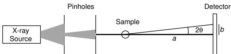
Figure 1.1: A SAXS camera with a point-collimated beam and a one-dimensional detector
