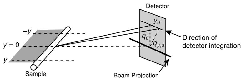
Figure 1.6: Contributions of different scattering angles due to integration along the width of the the detector.
