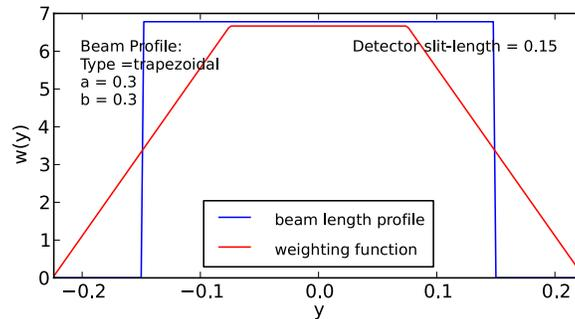
Figure 1.11: Weighting function for a rectangular beam profile, with (red) and without (blue) additional smearing due to integration over a detector slit width of  $0.15 \text{ \AA}^{-1}$
