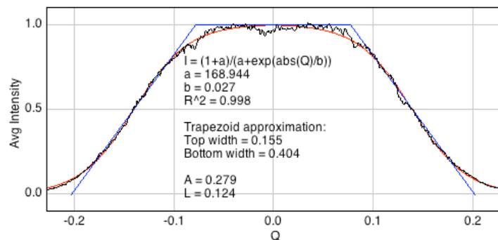
Figure 1.8: A fit of the sigmoidal function to a measured beam-length profile. From ImageJ with the saxsImage plugin.
