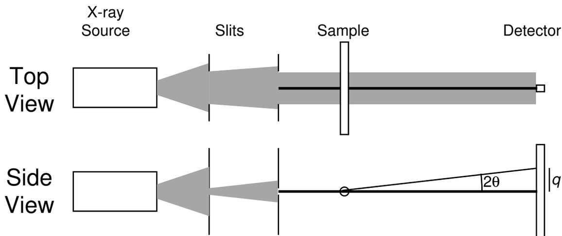
Figure 1.3: A SAXS camera with a line-collimated beam
