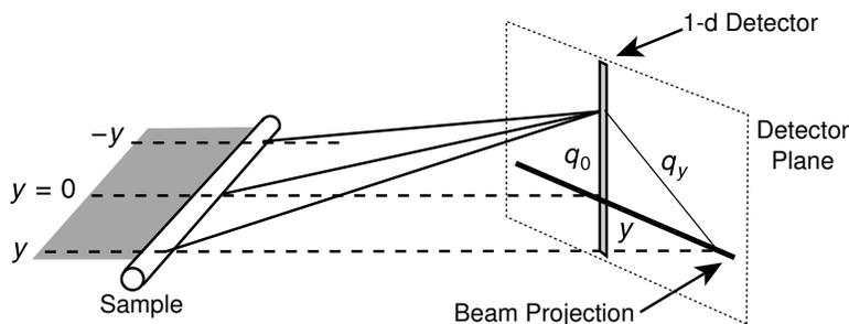
Figure 1.4: Contribution of X-rays scattered from multiple points along the beam length to the intensity detected at point  $q_0$ .
